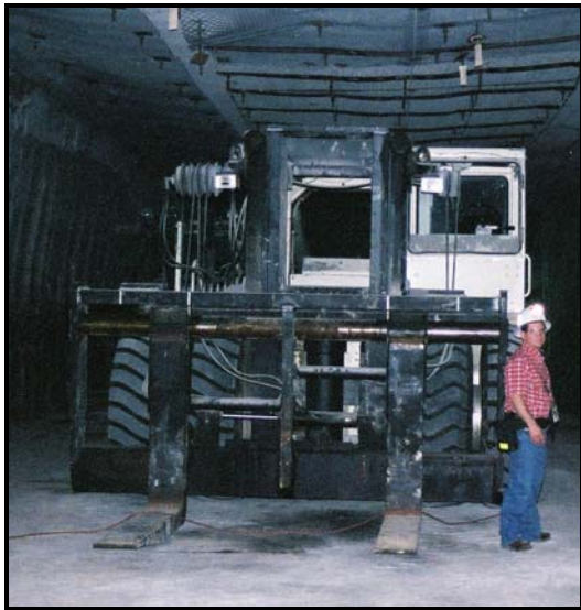
Figure 10-3 – 41 ton Forklift at WIPP (Courtesy: WIPP)
